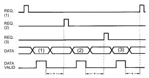
\*The period between the DATA VALID signal and the REQ signal should be no less than 20 ms max.
