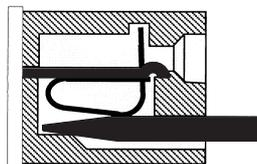
2. Insert the exposed conductor into the wire connection hole.
