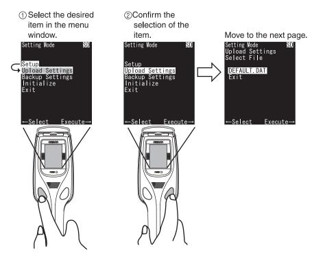
This series of operations whereby pressing the left trigger button to select [Upload Settings] and then pressing the right trigger button to confirm the selection is expressed as "selecting [Upload Settings]".
