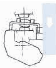
2. When contacts are being pulled apart.
