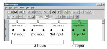
**Note** On the ZEN Support Software displays, bits in the ZEN memory are called "relays," program input bits are called "contacts," and program output bits are called "coils."
