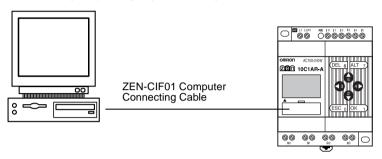
Note The connector on the computer side of the ZEN-CIF01 Computer Connecting Cable is a 9-pin D-sub connector. When connecting to a computer that does not have a serial port, connect an RS-232C-USB Conversion Cable to the ZEN-CIF01 Computer Connecting Cable. An OMRON CS1W-CIF31 Conversion Cable can be used (cable length: 50 cm).
