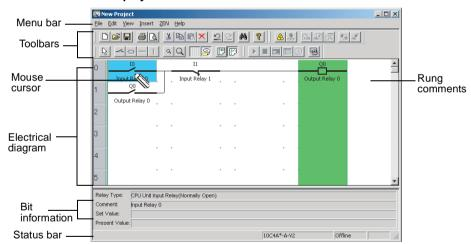
Note To switch between the ladder diagram and electrical diagram displays, either click on the buttons in the Toolbar or else select View(V)/Circuit display method/Ladder rung diagram/
