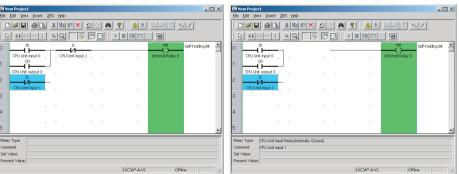
Note Either the pencil or arrow cursor can be used to copy, cut, and paste individual objects.
