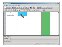
The Edit Input Dialog Box will be displayed again. Specify the bit type, type of input, bit number, and enter a comment if required, just as you did in step 4.
