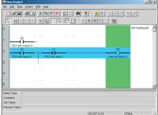
Note A program saved in a ladder program file can be pasted after copying the program and then starting up the ZEN Support Software in a separate window.
