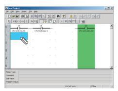
The Edit Input Dialog Box will be displayed. Specify the bit type, type of input, and bit number, and enter a comment if required, just as you did in step 4.
