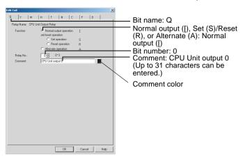
Move the mouse to the input position on the next line and doubleclick.
