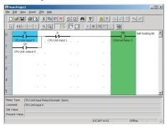
Note Connection lines cannot be drawn while the **Select objects** Button on the Toolbar is pressed. To return to
