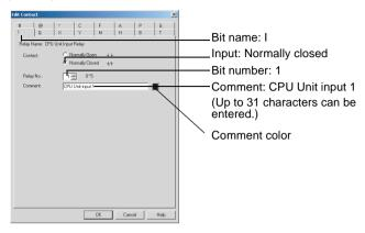
Move the mouse to the output bit position and double-click the mouse.
