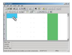
Note Input positions for input and output bits can be set by using the mouse or cursor keys to move to the input or output position and then use any of the following methods.
